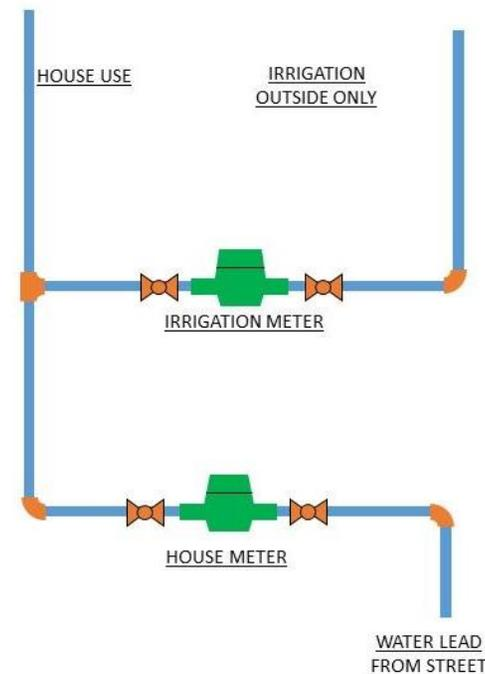
*Second (Irrigation) Meter Plumbing Diagram*
